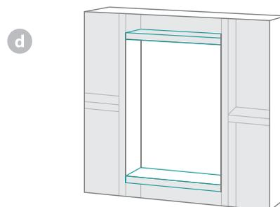
Remove the mirror cabinet door(s) by removing the screws on the door (not the screws on the cabinet body) and set aside, then position the mirror cabinet into place. Verify that the cabinet is level; use shims to adjust as necessary. See figure (e).
