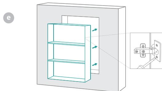
When the cabinet is in the proper position, secure to the wall with the provided mounting hardware (drill pilot holes for the screws if needed). See figure (f).
