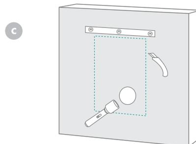
When the installation hole has been cleared of all obstructions, securely attach horizontal noggins to the vertical wall studs to create framing for your cabinet. Ensure the plaster wall edge is secured to the wall studs. See figure (d).
