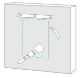
When the installation hole has been cleared of all obstructions, securely attach horizontal noggings to the vertical wall studs to create framing for your cabinet. Ensure the plaster wall edge is secured to the wall studs. See figure (d).
