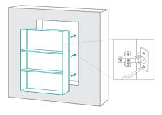
When the cabinet is in the proper position, secure to the wall with the provided mounting hardware (drill pilot holes for the screws if needed). See figure (f).
