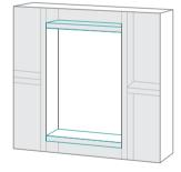
Remove the mirror cabinet door(s) by removing the screws on the door (not the screws on the cabinet body) and set aside, then position the mirror cabinet into place. Verify that the cabinet is level; use shims to adjust as necessary. See figure (e).
