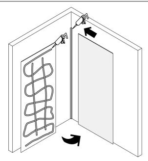
Use a generous amount of adhesive or silicone on the back side of the panel. Apply a 5mm bead of silicone to the inside of the trim from top to bottom. Slide the panel into the trim to secure it to the wall. Apply gentle, even pressure on the front of the panel to secure it in position.
