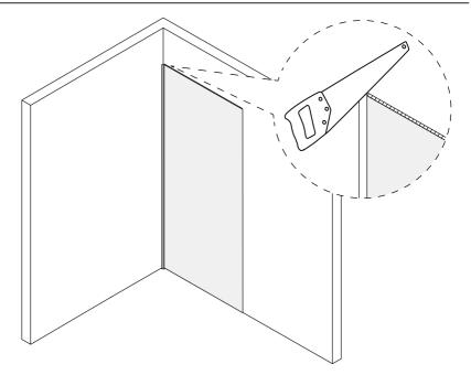
Use a fine tooth saw to cut off the tongue and groove part from end of the panel that will be placed inside the corner trim. Repeat this step for installing any edge trims at the end of the panel span.
