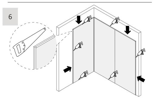
Measure and cut edge trim according to the requirement. Top edge will need to be trimmed to fit against corner and side edge trims. Run a bead of silicone along inside of the trim to secure it into place. Finally, run a bead of silicone along the complete bottom of panels and around any plumbing.
