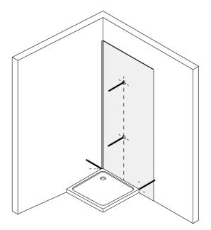
Before fixing any panel or trim, accurately measure and mark out the required pluming cutouts and other size adjustments if required. Carefully cut the panels and trims using a fine tooth saw or utility knife. For plumbing cut outs use a drill with a hole saw drill bit.
