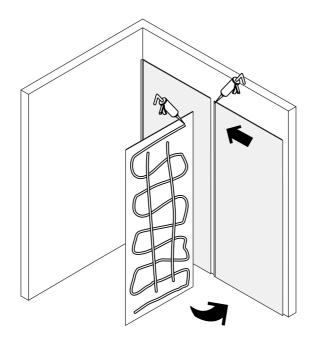
To install an adjoining panel use the tongue and groove connection between panels. Place adhesive on back side of panel and run a 3mm silicone bead down the groove before connecting the panels.
