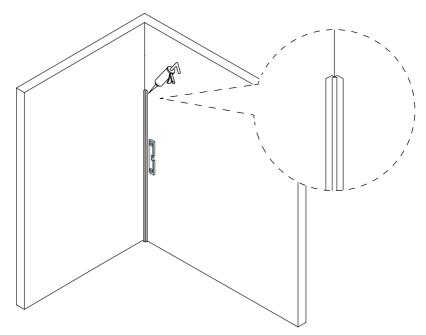
Run a silicone bead running all the way down both back sides of the corner trim to secure it to the supporting wall. If installing over a shower base, measure and cut the corner trim accordingly.
