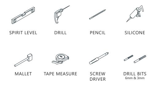
Required drill bits are 6mm & 3mm (1/4" & 1/8")Use a 6mm (1/4") drill bit for ceramic when drilling into ceramic tiles.
